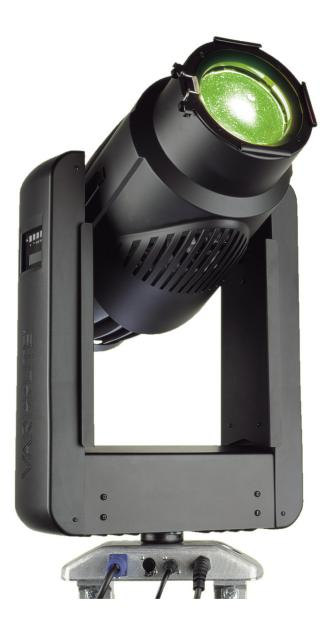
The Vari-Lite VL1100 luminaires have a 50kHz drive system that quietens the operation of all two-phase motors in the fixtures during movement and while in static positions. They also have three-phase, ultra quiet stepper motors that provide a smooth, timed continuous pan and tilt motion. Additionally, a central bearing system in the gobo wheel reduces noise and ensures smooth operation.
