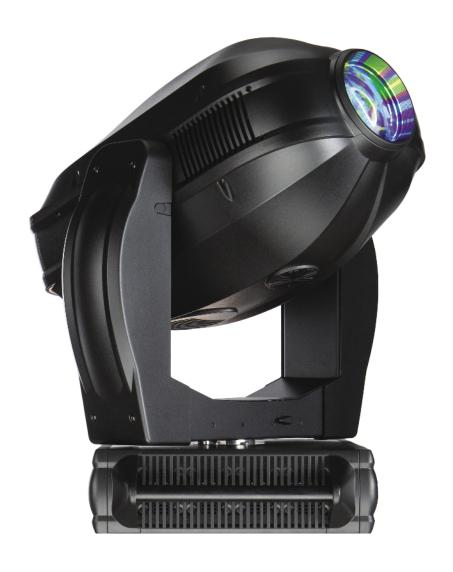
Every aspect of the Vari-Lite VL4000 Spot luminaire has been designed with performance in mind using a Philips 1200W lamp to produce 33,000 lumens in standard mode (25,000 studio mode) and high resolution optics to ensure remarkable center-to-edge focusing, with a 5:1 zoom that covers an amazing 9 to 47 degrees without sacrificing output or clarity.
